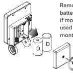
Remove D Cell (LR20) batteries from the PM5 if monitor will not be used for a period of four months or more.
