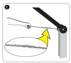
1. Do not use if drive cord shows excessive signs of wear
