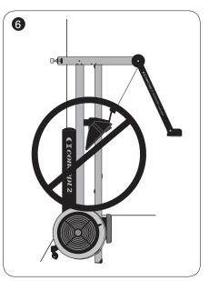
6. Do not leave the Dynamic Indoor Rower unattended in a standing position. Stand it up only for access to machine for maintenance.
