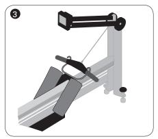
3. Place handle in the foot carriage handle hook whenever the machine is not in use.
